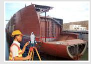
Large shipbuilding surveying and positioning
