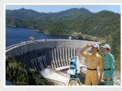
For target within 500m, prisms are not required. The surveying work is easily finished
