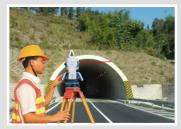
**Tunnel Measurement** Be able to observe measuring point without prisms. Pointlayout becomes easier
